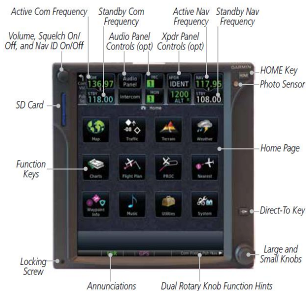
Figure 1- GTN 750 Control and Display Layout
